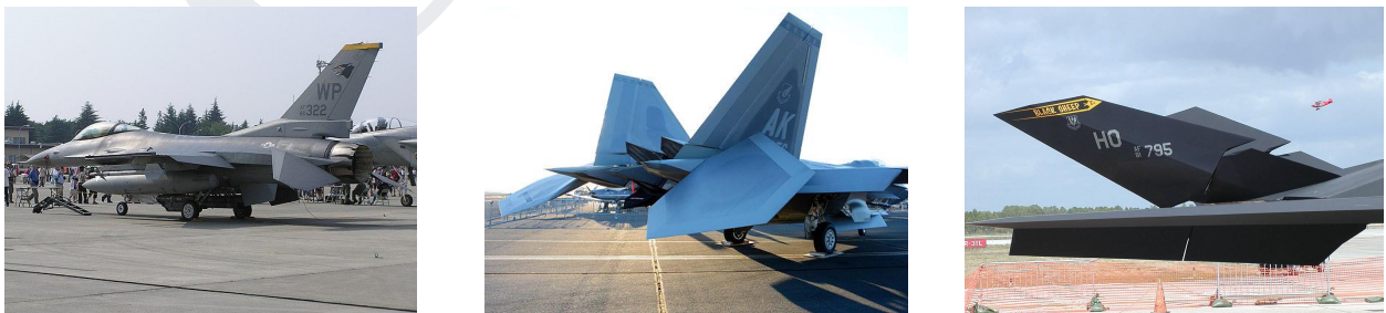
Fig. 29. Examples of stabilators, tailerons and ruddervators.
