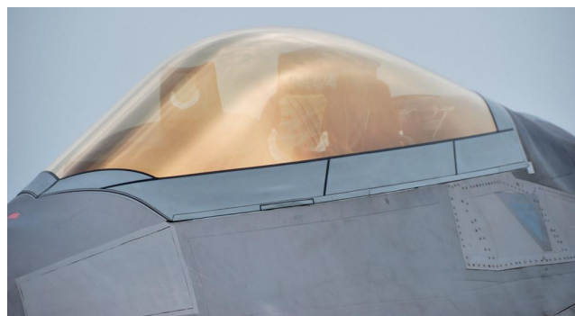
Fig. 90. F-22 canopy glass showing stealth coating.
