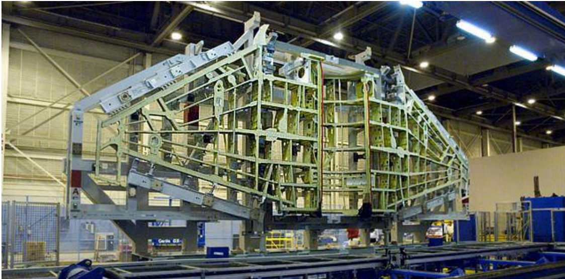
Fig. 161. F-35 wing structure, courtesy of Lockheed Martin.
