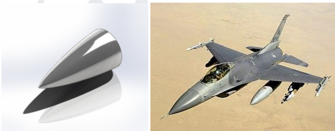
Fig. 36. Von Karman nose cone shape.
