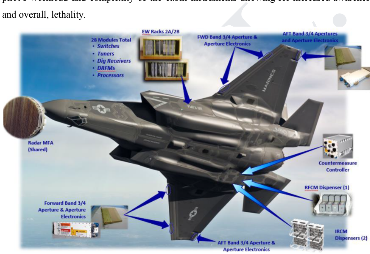
Fig. 97. Electronic warfare modules and their position within the F-35 airframe, courtesy of www.Aircraft101.com .
