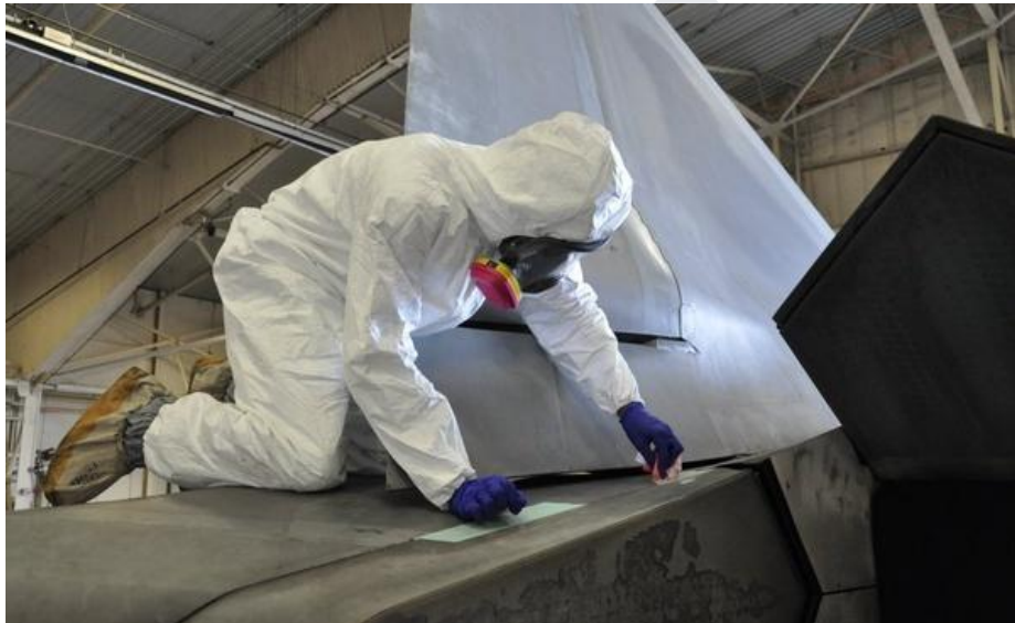
Fig. 95. Maintenance operations in the F-22’s stealth coating, courtesy of Lockheed Martin.
