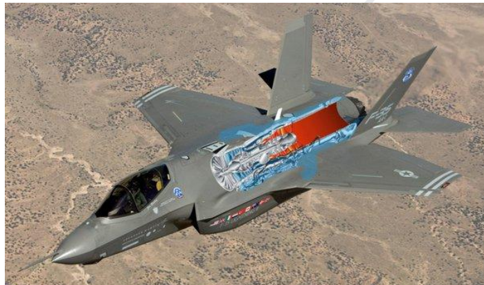
Fig. 93. F-35 method of IR signature reduction.
