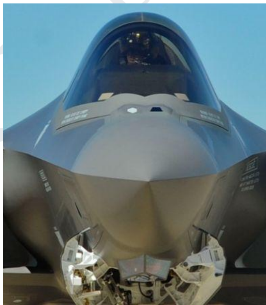
Fig. 99. F-35 front view. Top: IRST module part of Northrop Grumman’s AN/AAQ-37 360° view system. Bottom: Lockheed Martin’s EOTS, intended for ground targets.
