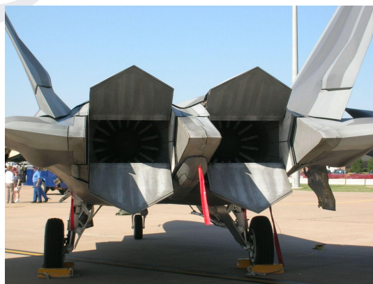
Fig. 94. F-22 rectangular nozzle design.
