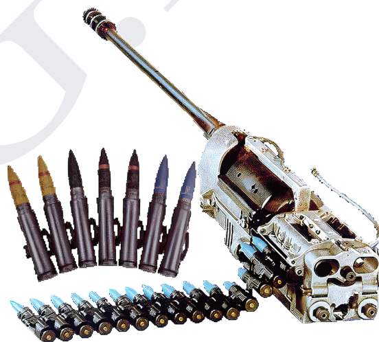
Fig. 78. Mauser BK-27 revolver cannon and feeding system.
