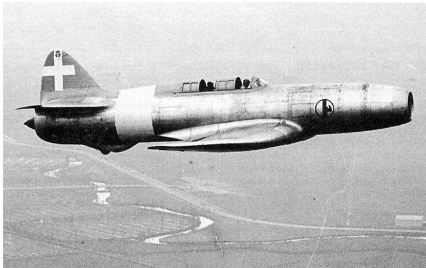
Figure 2.2. Campini Caproni C.C.2, 1940, early jet engine, WWII Italy (Phil DeFer).
