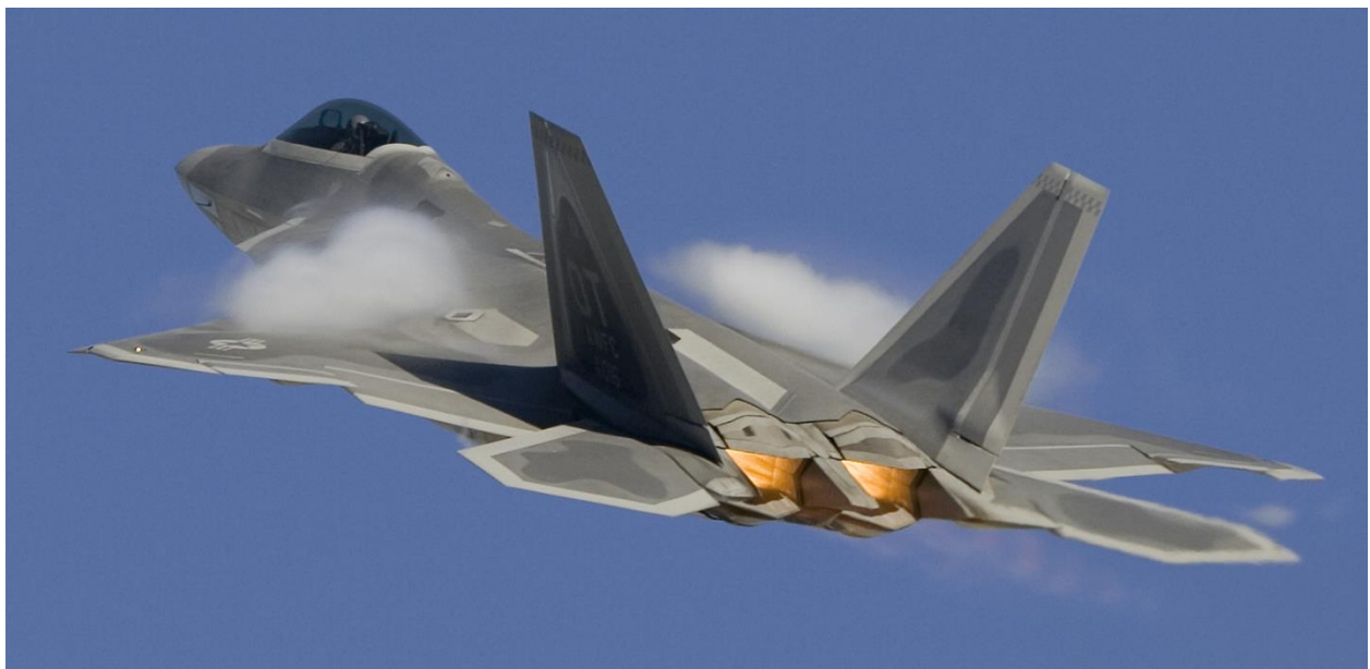
Figure 2.8. Bi-Dimensional exhaust nozzle fitted onto the F-22 Raptor.
