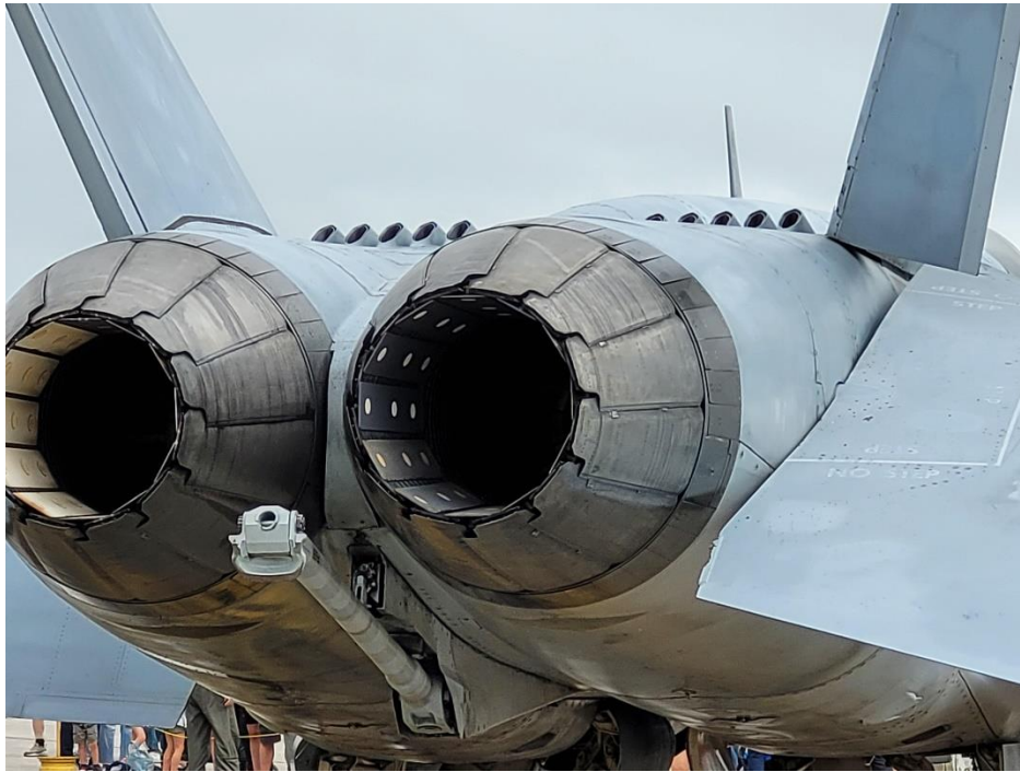
Figure 2.7. Axisymmetric exhaust nozzle fitted onto the F/A-18 Hornet.
