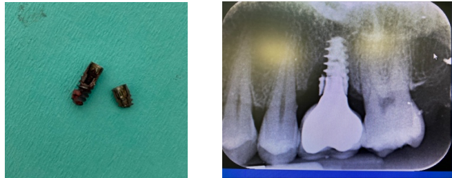
Figure 5 and 6: Pictures of implants fractured at the connection (Annex 1)
