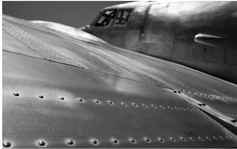
Figure 1.2: Aircraft skin with riveted joints
