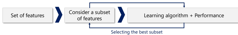
Figure 3.9: Pipeline scheme for the implementation of embedded feature selection methods.
