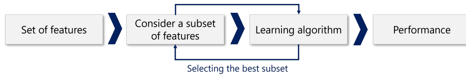
Figure 3.8: Pipeline scheme for the implementation of wrapper feature selection methods.
