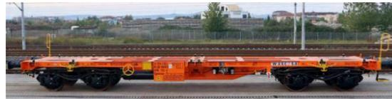
Figura 28: Wascosa 40' container flat wagon, Sgmms
