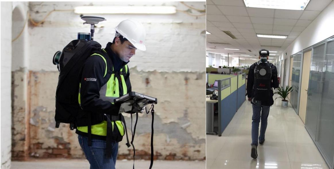
*Ilustración 62. Leica Pegasus: Backpack. (Leica Geosystems., 2019)*
