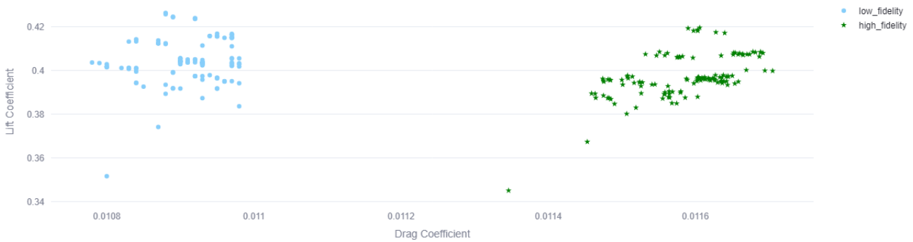
Figure 35: C_L vs. C_D of XFOil results and their respective Star-CCM+ results of PARSEC geometries.
