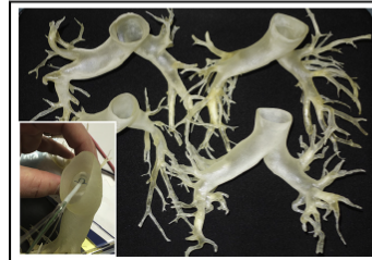
Flexible 3D printed models with inset, showing their use testing a catheter prototype.
